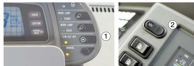
1:T/M cut-off ON/OFF switch 2:T/M cut-off set switch
