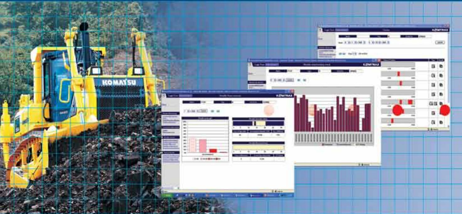
KOMTRAX is Komatsu's remote equipment and fleet monitoring system. Leading-edge wireless technology and a secure, user-friendly, Web-based application provide critical information . . . anytime, anywhere.
