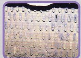
Scales are completely clogging the radiator.
