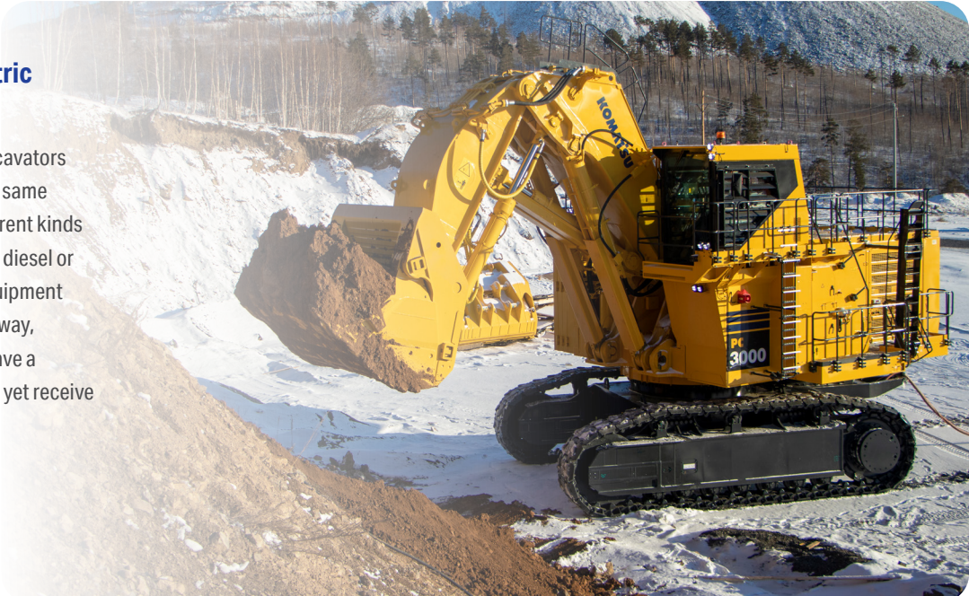
Calculations were done with the standard bucket capacity, 85% of bucket fill factor and 1.8 ton/m 3 density.
